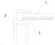
The depth is no less than 3mm when installing the module into the frame.
