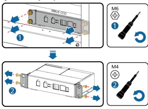
Figure 7-6 Removing a faulty SmartMBUS CCO module
