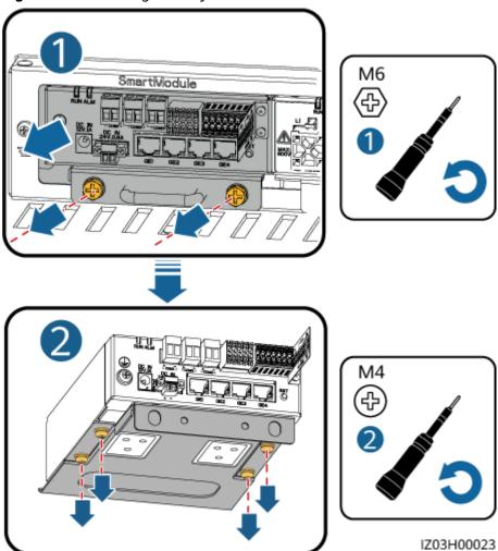
Figure 7-9 Removing a faulty SmartModule
