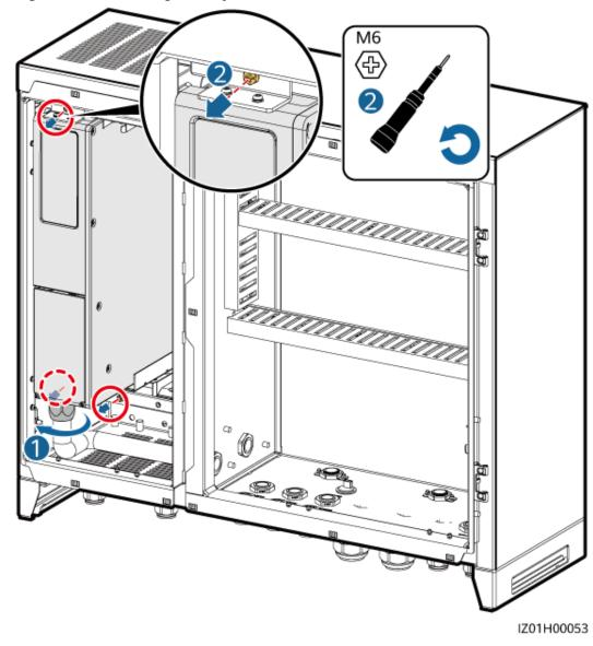
Figure 7-14 Removing a faulty PID module
