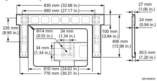
Figure 4-2 Mounting bracket dimensions
