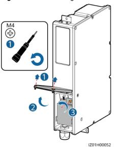
Figure 7-13 Removing the cover from a connection box
