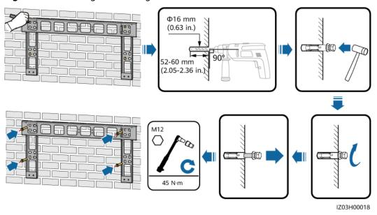
Figure 4-3 Installing a mounting bracket
