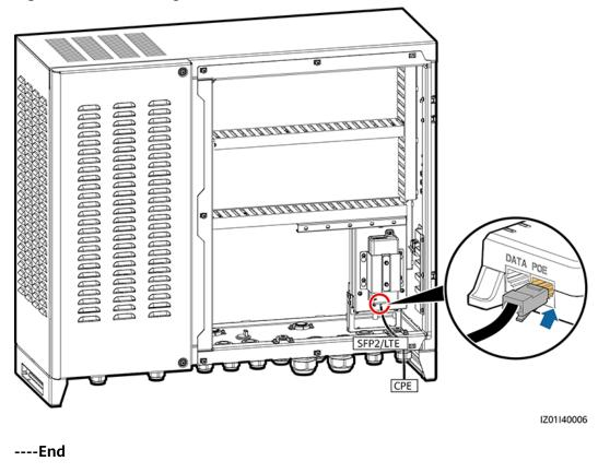
Figure 5-15 Connecting a CPE network cable
