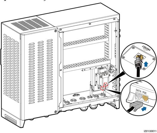
Figure 5-11 Connecting a PoE module to a PoE SPD
