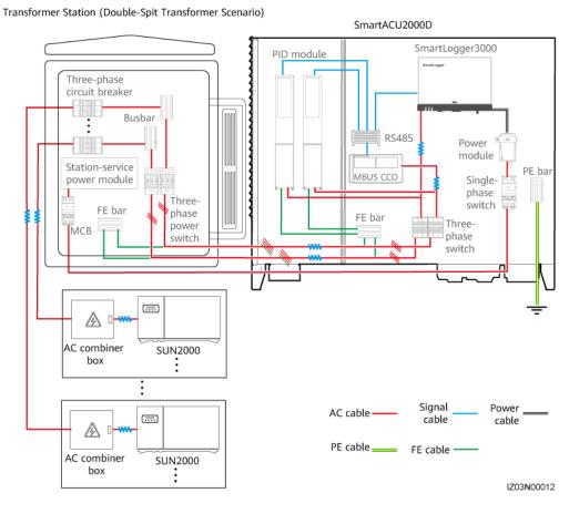
Figure 2-9 MBUS communication mode
