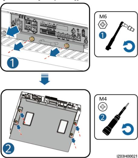
Figure 7-7 Removing a faulty SmartLogger
