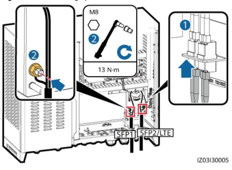
Figure 5-10 Connecting optical cables
