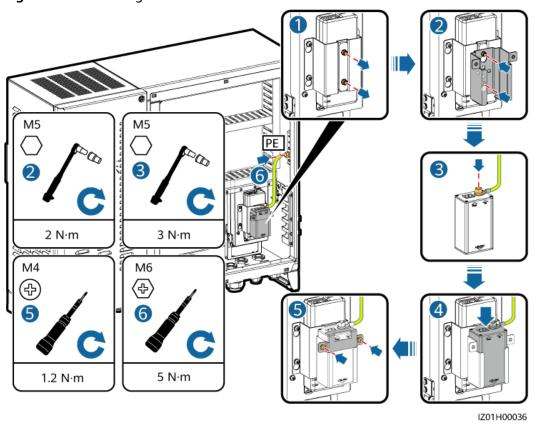
Figure 4-14 Installing a PoE SPD
