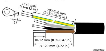
Figure 5-16 Length for cable stripping
