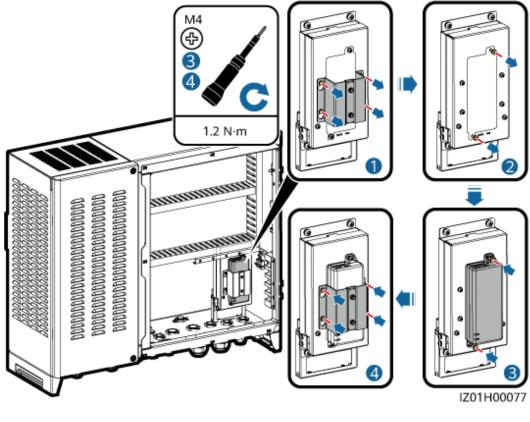
Figure 4-13 Installing a PoE module
