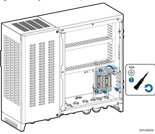
Figure 5-8 Removing external mechanical parts
