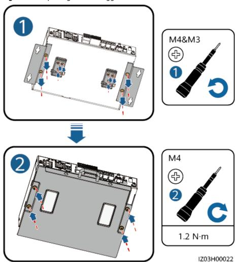
Figure 7-8 Replacing a SmartLogger
