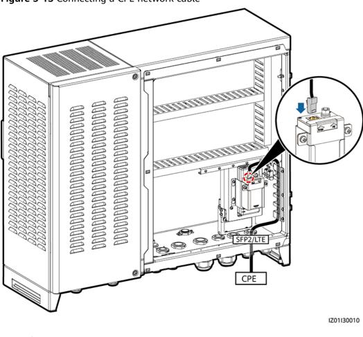
Figure 5-13 Connecting a CPE network cable
