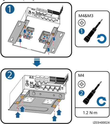
Figure 7-10 Replacing a SmartModule
