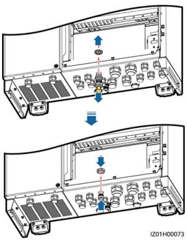
**Step 3** Route the cable through the pipe conduit and then the fitting, and connect the cable.
