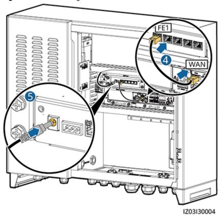
Figure 4-11 Connecting cables to an Ethernet switch
