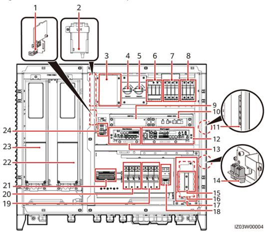
Figure 2-5 SmartACU2000D-D-03 components
