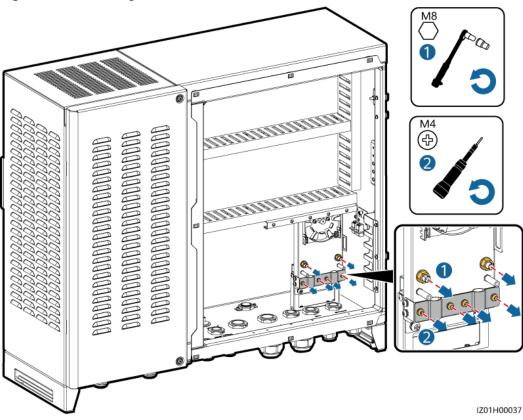
Figure 5-9 Removing a fastener
