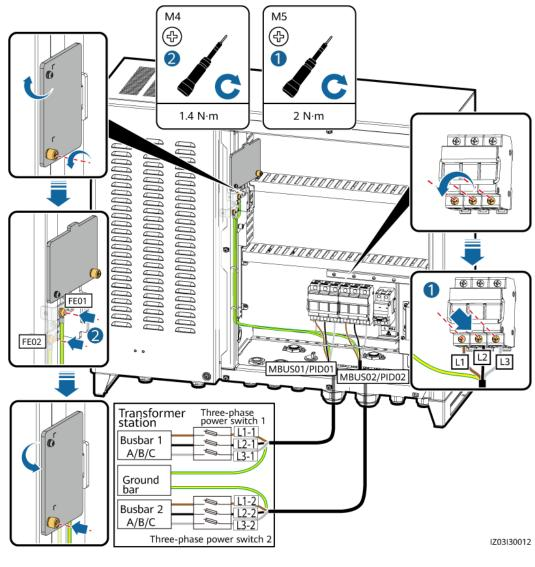
Figure 5-17 Connecting a cable
