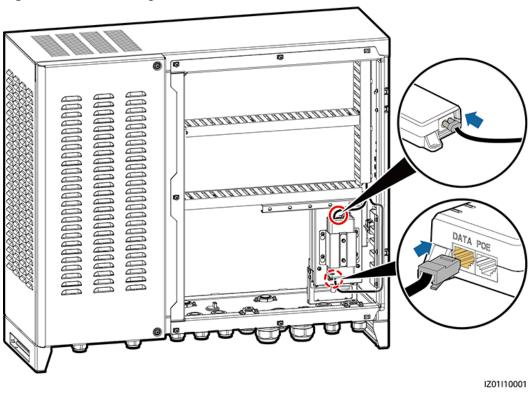
Figure 5-14 Connecting cables to a PoE module
