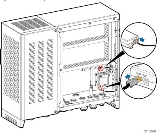
Figure 5-12 Connecting cables to a PoE module
