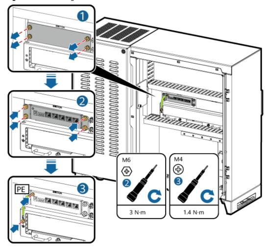
Figure 4-10 Installing an Ethernet switch
