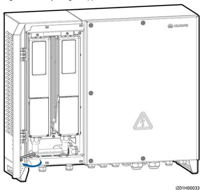
Figure 7-12 Adjusting a support bar
