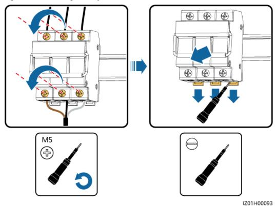
Figure 7-3 Removing a faulty knife fuse switch
