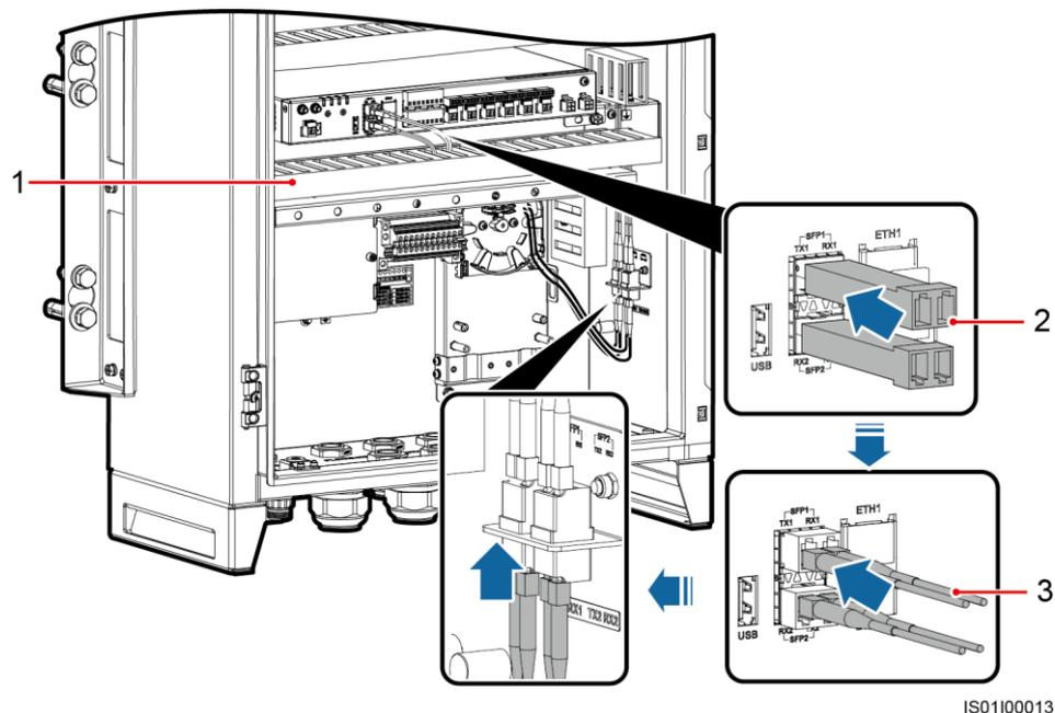
(1) Cable trough for the factory-installed optical jumpers
