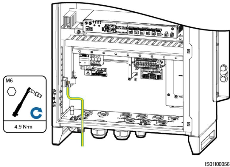
**Figure 5-4** Connecting a PE cable (through a pipe)
