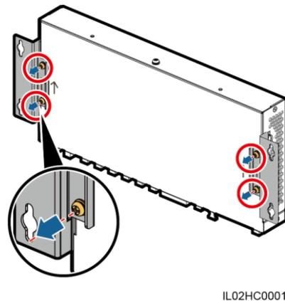
**Step 4** Remove the mounting bracket from the faulty SmartLogger2000 and install it on the new SmartLogger2000.
