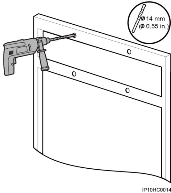
**Step 3** Insert the M12x60 bolts (expansion bolts with only flat washers and spring washers) into the holes, and secure them using the delivered nuts and flat washers.
