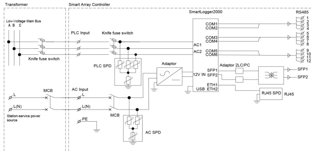
The smart array controller communicates with the inverter over PLC and communicates with the central control room over a fiber ring network.
