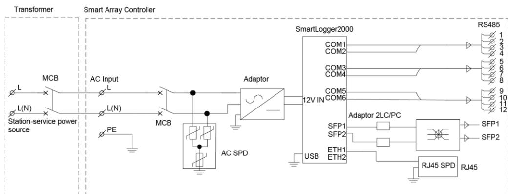
The smart array controller communicates with the box-type transformer and inverter over RS485 and communicates with the central control room over a fiber ring network.
