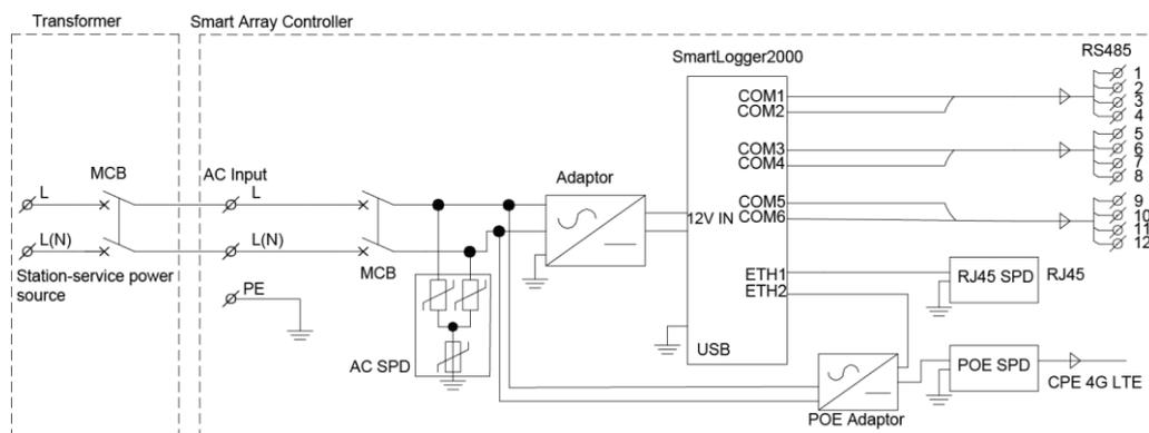
The smart array controller communicates with the box-type transformer and inverter over RS485 and communicates with the central control room over 4G LTE.
