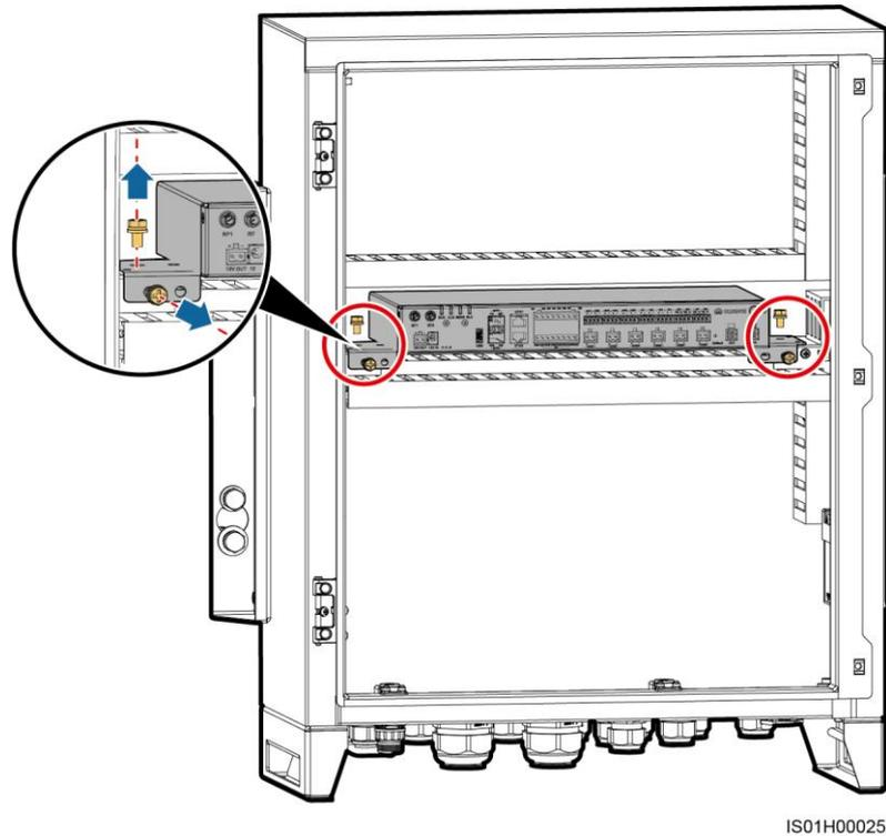
**Step 3** Remove mounting ears from the new SmartLogger2000.
