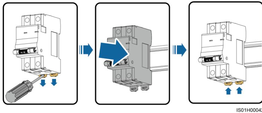
**Step 4** Reconnect the cables to the single-phase power switch based on the cable labels.
