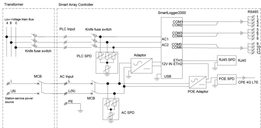
The smart array controller communicates with the inverter over PLC and communicates with the central control room over 4G LTE.
