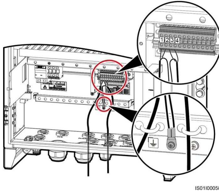
**Figure 5-18** Connecting RS485 communications cables (through a pipe)
