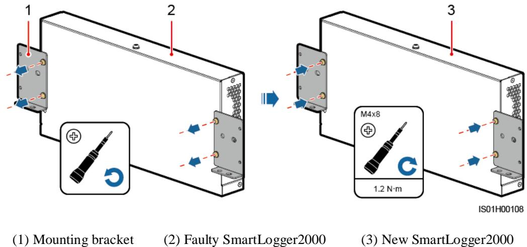
**Step 5** Install the new SmartLogger2000 in the smart array controller.
