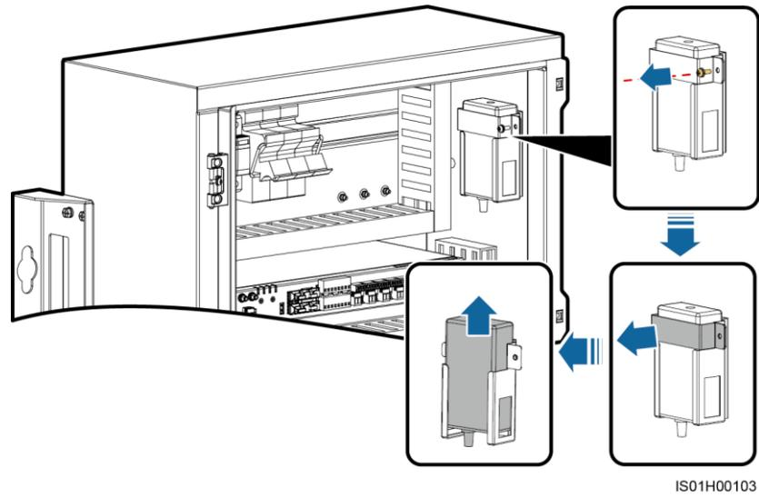
**Step 3** Install the new power adapter.
